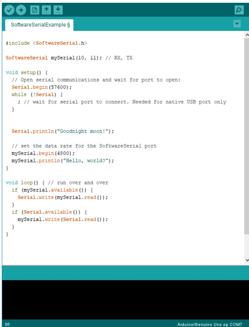
The screenshot shows the Arduino IDE interface with the 'SoftwareSerialExample' sketch open. The code implements a SoftwareSerial port on pins 10 and 11, sets the data rate to 4800 bps, and performs a simple communication loop where it prints "Hello, world?" and reads from the serial port. The IDE status bar at the bottom indicates the connection is to an 'Arduino/Genuino Uno' on 'COM7'.
